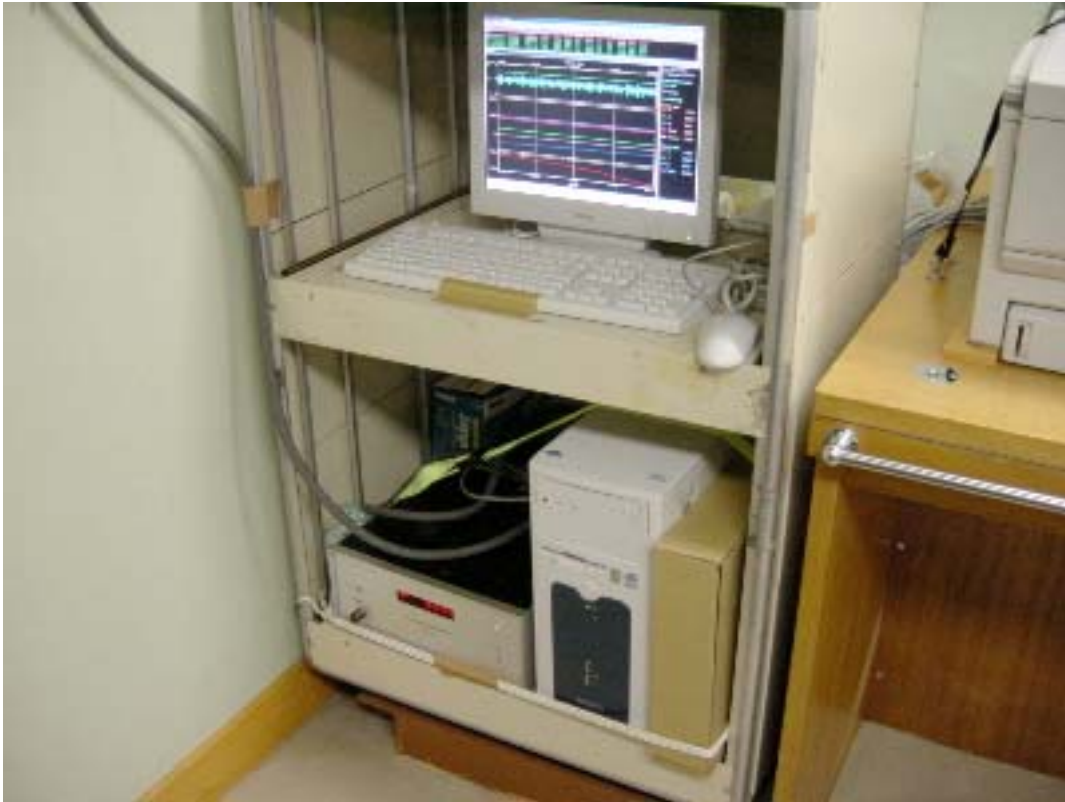
Figure 13 SBM-89 settled in NO.1 Laboratory. The controll unit of the magnetometer is on lower of the rack, and the computer records magnetic data merged with ship's navigation and motion data.
