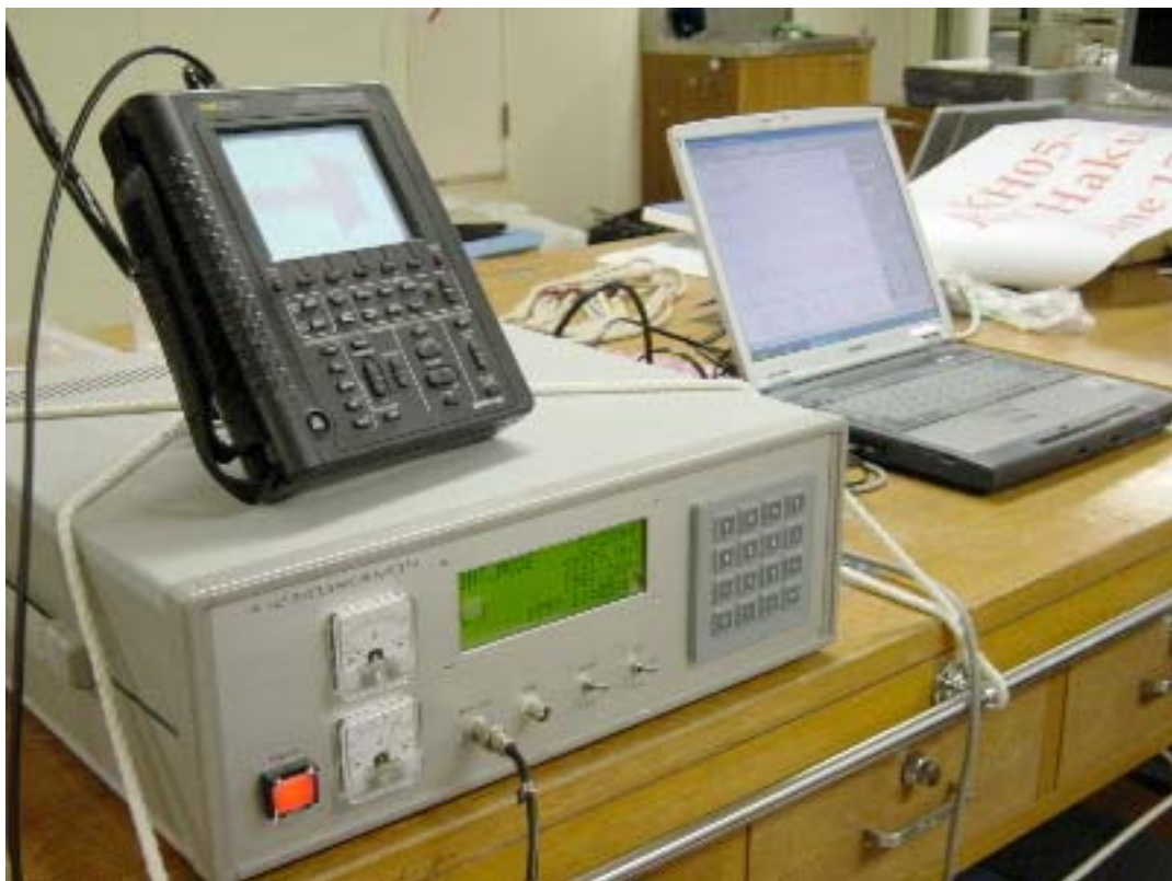
Figure 10 PR-745 proton precession magnetometer settled in NO.3 Laboratory. The controll unit of the magnetometer is in the left-hand of the photograph, and the computer in the right-hand records magnetic data merged with ship's navigation data.
