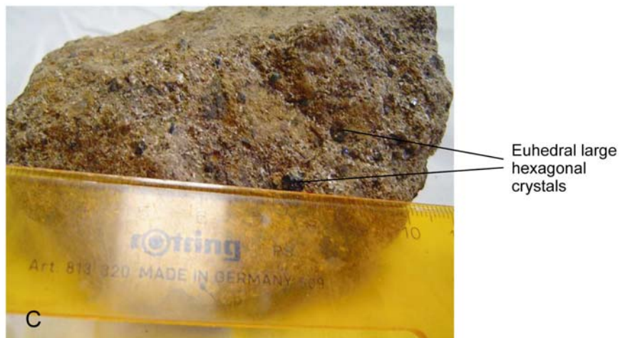
Figure 24 Close-up photos of the samples from dredge D1. (A) Heavily weathered pillow basalt. (B) Coarse-grained suspicious plutonic rock. (C) Very large grain of euhedral pyroxene or hornblende (maximum ~ 5 mm in length) in coarse-grained suspicious plutonic rock.
