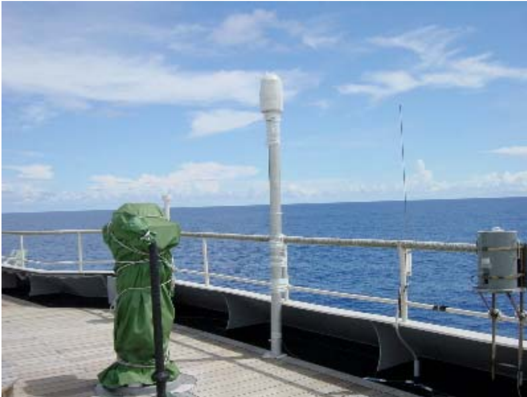
Figure 14 The fluxgate sensor of SBM-89 is settled on the upper deck above the bridge.
